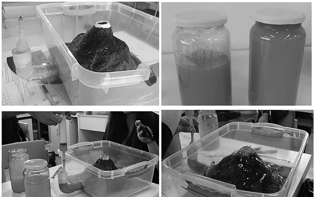
Figure 3. Analog model of volcanoes. Mixtures with different viscosities are pushed out and through the top of the volcano. It is possible to compare, how the slightly viscous and very viscous mixtures descend from the top.
